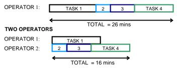
Figure 4: Operators influence on changeover time The influence of the number of operators on the changeover is depending heavily on the tasks that have to be executed in a changeover, and thus on the 'From' and 'To' SKU. type of changeover. One of the tasks of the changeover model is that it detects the 'from' and 'to' SKU and then determines the tasks to be executed.
